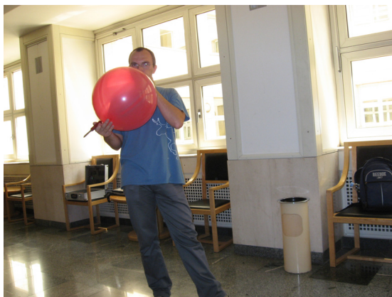
Fig.6. A balloon as an impulsive source
