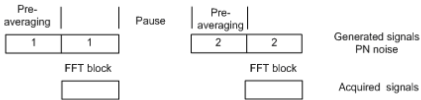
Figure 2.4 Signal generation and acquisition during the asynchronous frequency domain averaging
