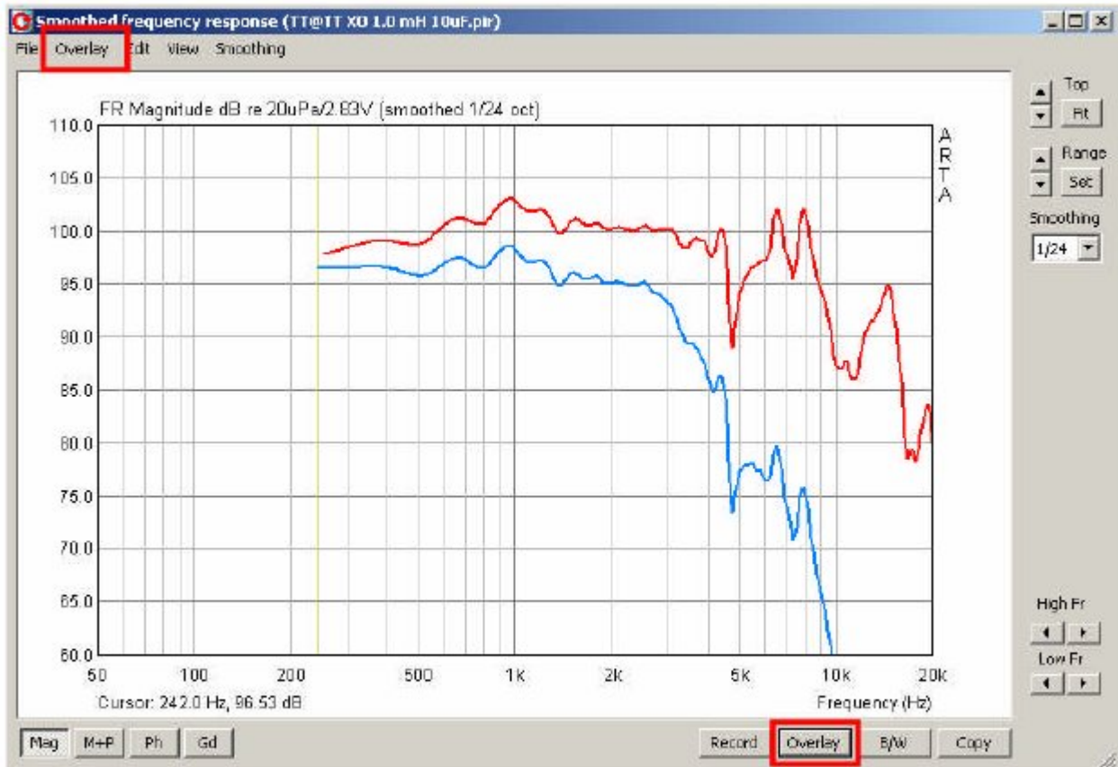
Figure 8.1.4 Smoothed frequency response window with overlay.
