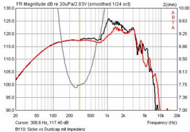
Figure 7.3.10 Surround frequency response (black), dust cap (red) and impedance (grey).
