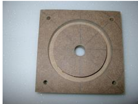
Figure 3.4 Front (interior) view with circular groove for pipe mounting
