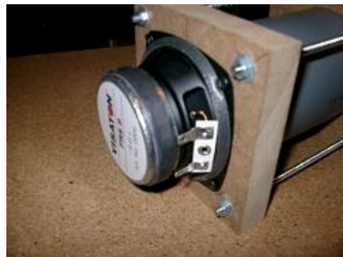
Figure 3.2 Rear view of the completed chamber with Visaton FRS8 driver
