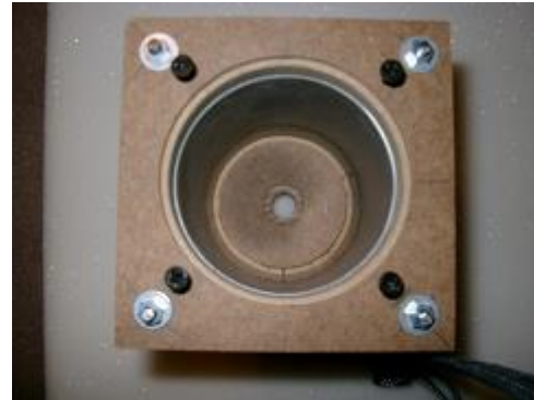
Figure 3.6 Rear panel (driver side), exterior view showing nut plates for mounting the driver
