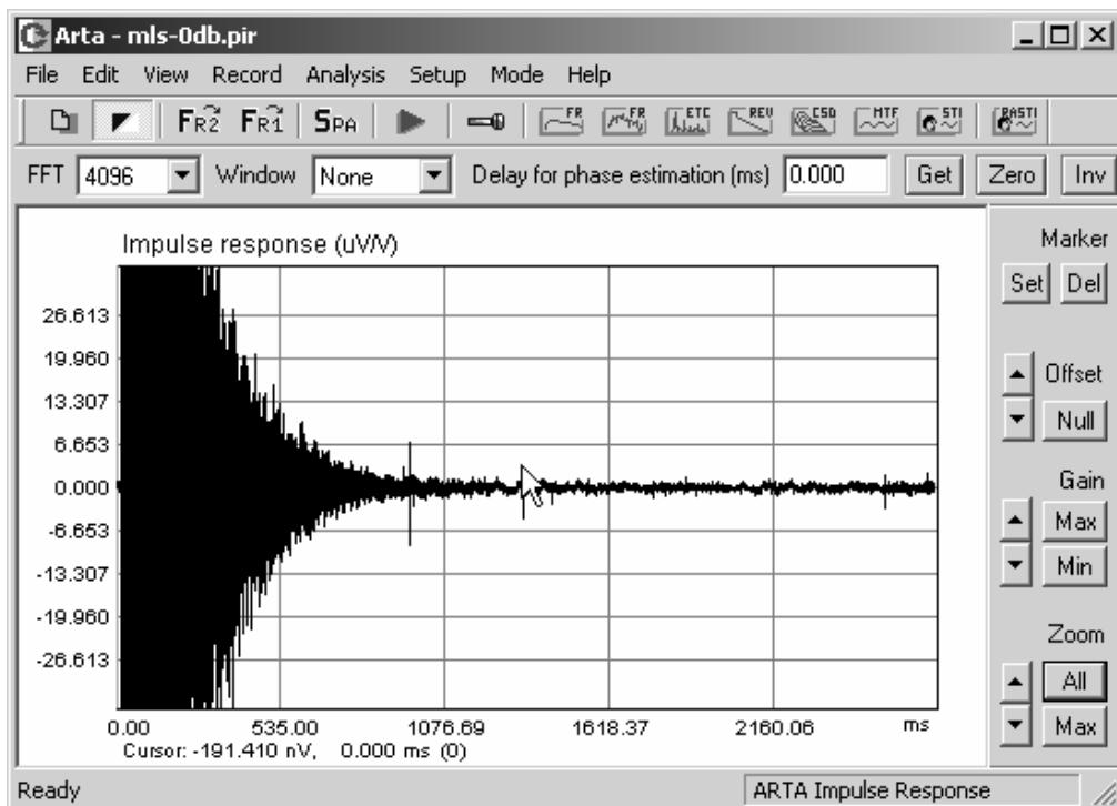
**Figure 1.** ARTA window for impulse response analysis (MLS-estimated PIR is shown)
