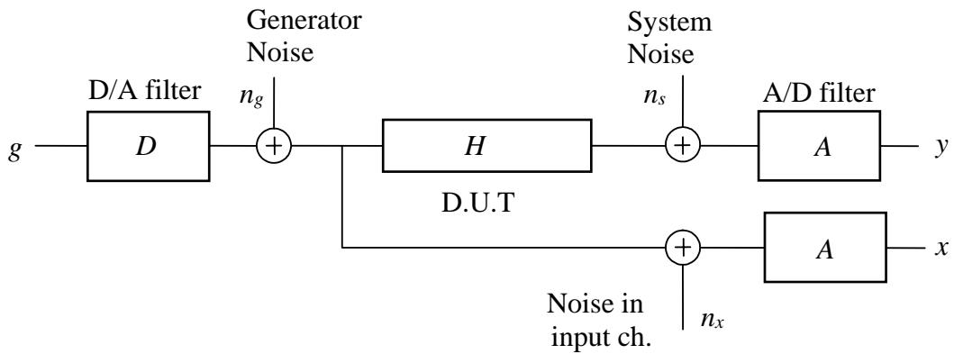
**Figure 2.** Block diagram of the measuring system
