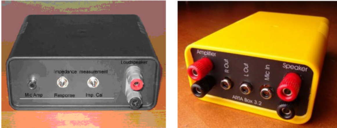
Figure 3.1 The finished measurement box (conventional wired version left, PCB version right).
