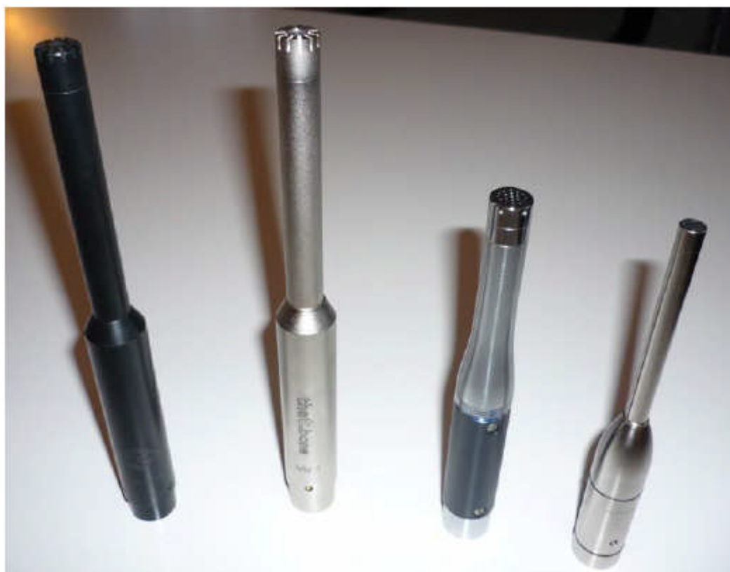
Figure 5.2.1 Measurement microphones (from left to right): Haun MB550, t-Bone MM1, NTI M2210, Audix TM-1.
