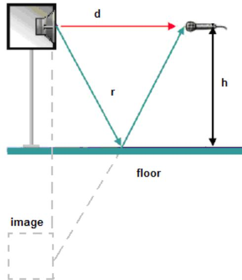
From the direct wave path length  $d$  and the distance  $h$  from floor we get the path length of the first reflection
