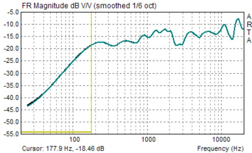
We save this curve as overlay. Cursor and yellow line at the bottom of the graph denote that the time-bandwidth requirement is satisfied on frequencies above 177.9Hz. (Note:  $1/\text{gate} = 1000/5.604 = 178.4$ )
